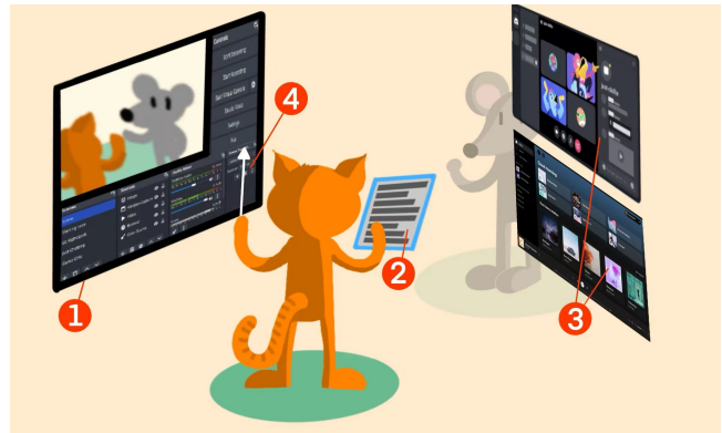
Figure 3: Examples of 2D window overlays social VR streamers need to manage for their streaming: (1) streaming manager (OBS) (2) audience chat, and (3) music and community software. (4) highlights the VR ray-casting control to navigate the menu items on 2D interfaces in VR.
